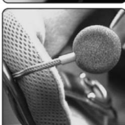
Apply light pressure around the outside edges to ensure that it adheres to the black fabric. Avoid squeezing the middle of the front and back covers as this can cause the microphone to move which may cause damage to the fine microphone wires.
