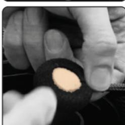
**Second:** Take one of the black velcro pads, remove the backing from the self adhesive velcro pad and apply it to the **BLACK** side of the microphone fabric.
