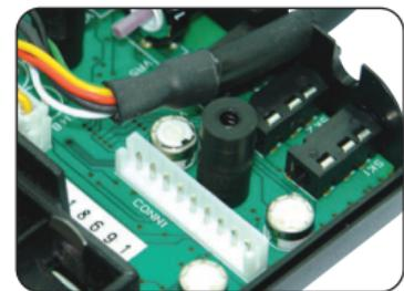
Carefully break off the blanking tab from inside the small back cover (the outer of the two, which previously covered one of the slots in the front panel) and then orientate the interface lead's white connector so that the red wire is towards the centre of the hub, before carefully aligning the pins and pressing the connectors together.
