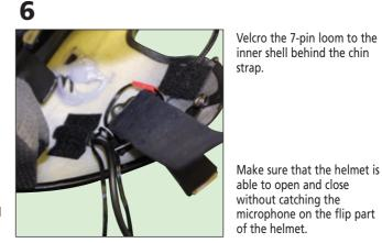
Velcro the 7-pin loom to the inner shell behind the chin strap.
