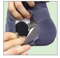
Place a small strip of velcro where the circle is. The speaker is then placed in the cheek pad in a vertical position with the wire to the bottom of the speaker. The wire is then placed through the chin strap hole. The fabric is put back in placed and taped back up in its original
