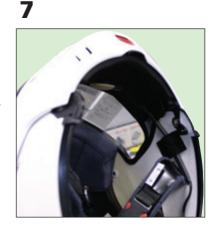
Once all this has been done, you are ready to put the helmet back together. Clip all the relevant clips together. The longer black wire with the white clip goes around the back of the helmet tucked away to the right hand speaker. Once the cheek pads are in position, make sure that the cheek pads clip back into the black clips.
