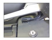
The passenger lead comes out near where the passenger sits and is positioned on the plastic near to the panniers.
