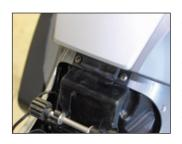
Remove the x2 T25 screws in the middle of the tank.
