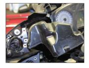
Pull out speakers to expose speaker wires behind.
